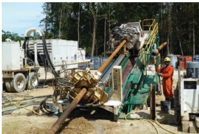
Plate 2.3 – Horizontal directional drilling rig in operation
