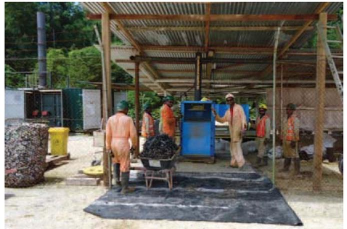
Plate 9.5 – Metal shavings being compacted into drums at Kopi Logistics Camp
