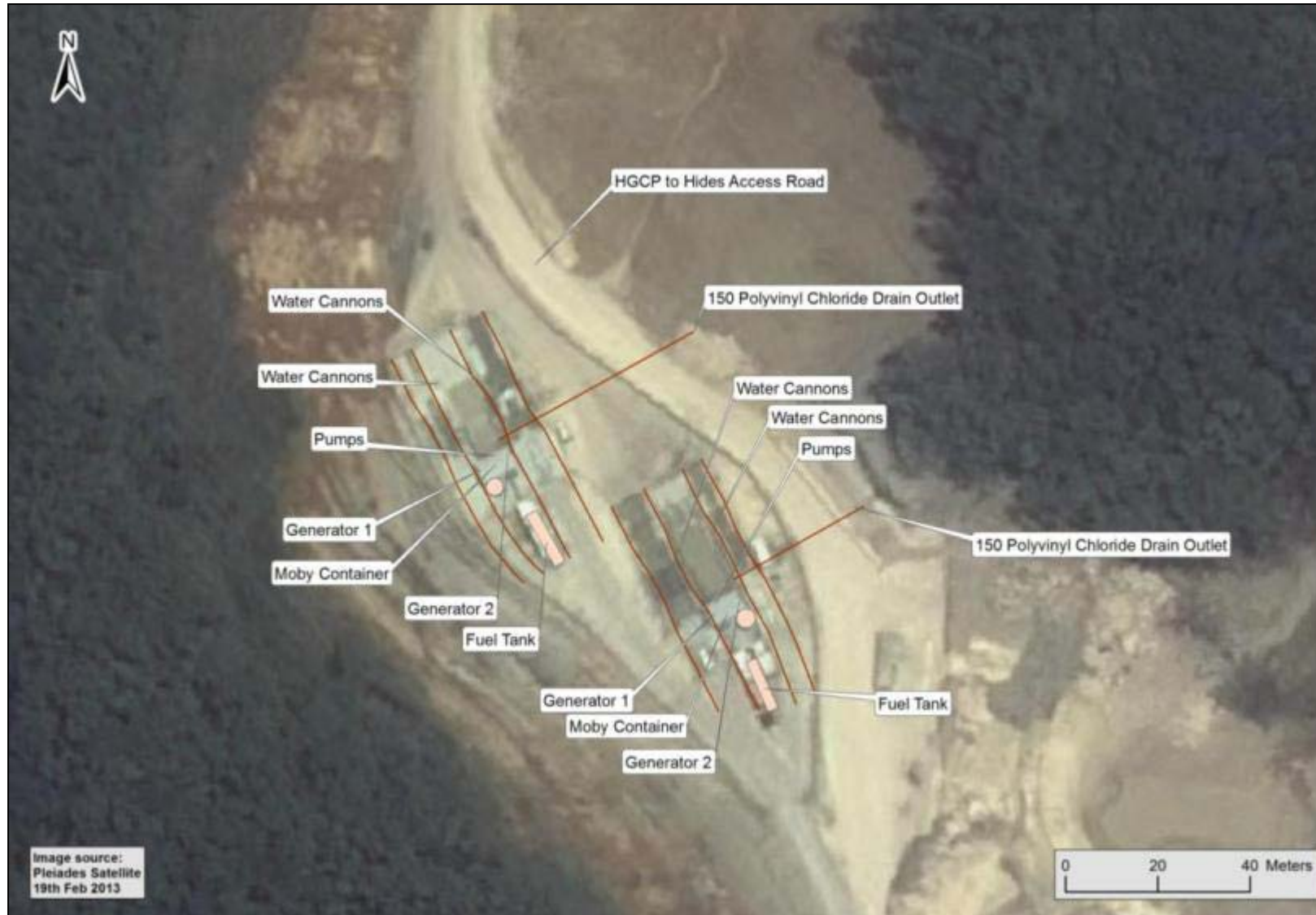
Figure 5-4: Hides Vehicle Wash Facility layout
